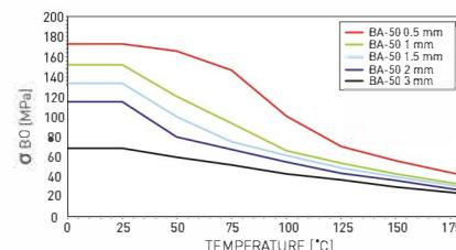
σ<sub>BO</sub> diagrams represent σ<sub>BO</sub> values for different gasket material thicknesses. These values indicate the maximum in-service compressive pressures which can be applied on the gasket area involved without destroying or damaging the gasket material.
