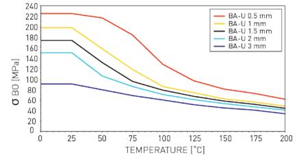
σ<sub>BO</sub> diagrams represent σ<sub>BO</sub> values for different gasket material thicknesses. These values indicate the maximum in-service compressive pressures which can be applied on the gasket area involved without destructing or damaging the gasket material.
