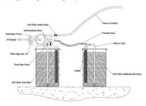
When the Void Filler has fully melted and the correct temperature reached proceed as follows:
