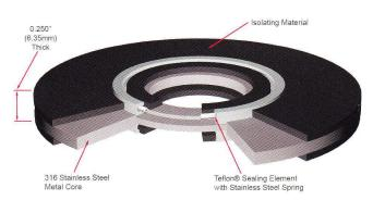
The DEFENDER™ sealing/isolating gasket system is designed for critical/extreme applications. Manufactured with a 316 stainless steel core retainer and laminated on both sides with high strength laminates, the DEFENDER™ gasket is resistant to deforming under load and is used when electrical isolation and corrosion control are required on pipes containing gas, natural gas, oil and other hydrocarbon based medias up to 392°F
